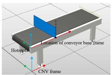
Locations along Y and Z of conveyor frame are determined by hotspot0.
