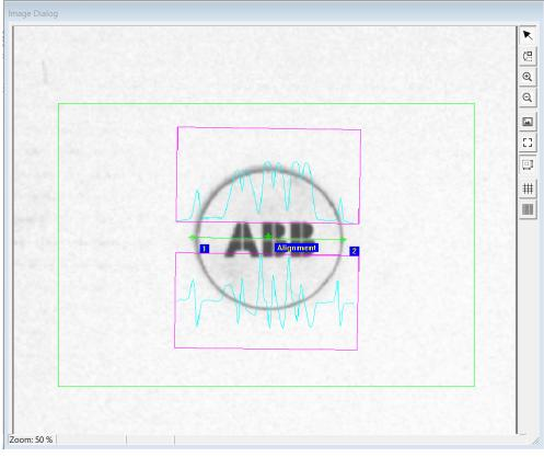
The checkboxes in the **Search parameter** define which results should be displayed in the **Image Dialog**.
