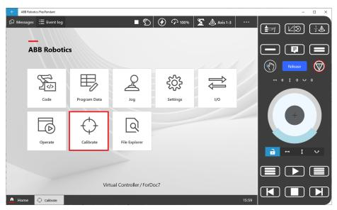
5 Open the Calibration window in Calibrate on the FlexPendant.
